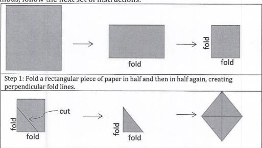
Step 2: Draw a line from anywhere on one fold to anywhere on the perpendicular fold. Cut along the line you drew. When you unfold, you will have a rhombus.
